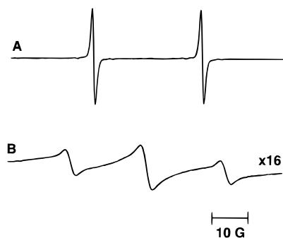
FIGURE 1: EPR spectra of (A) ^{15}\text{N} -TPL, 0.5 mL of 0.5 mM solution containing 5% human serum albumin, and (B) 0.5 mL of PNA in Ringer's lactate buffer. The concentrations correspond to those used in the heart experiments. Spectrum B, which is displayed at 16-fold higher gain relative to spectrum A, is asymmetrically broadened due to immobilization of the nitroxide residues bound to albumin. The instrumental settings were as follows: modulation field, 0.20 G; time constant, 20 ms; scan time, 10 s; modulation frequency, 100 kHz; microwave power, 15 mW; microwave frequency, 1.20902 GHz.
